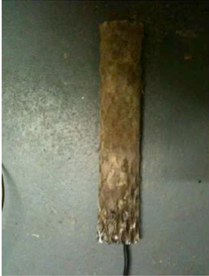
**Fig. 14 Zinc anode after 6 months of operation.**
